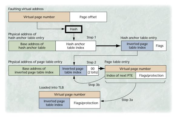
average collision-chain length by half, without having to change the size of the inverted page table. Since the entries in the hash anchor table are smaller than the entries in the inverted table, it is more memory efficient to increase the size of the hash anchor table to reduce the average collision-chain length.
