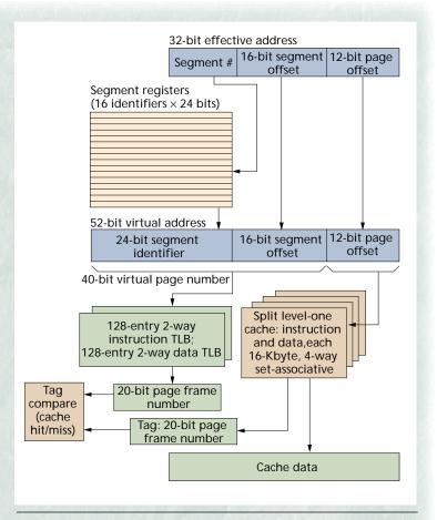
Figure B. The PowerPC 604 uses a hardware-managed TLB and a variant on the inverted page table—an eight-way software cache for PTEs. The cache index is the same size as the page offset, effectively making the caches physically indexed.
